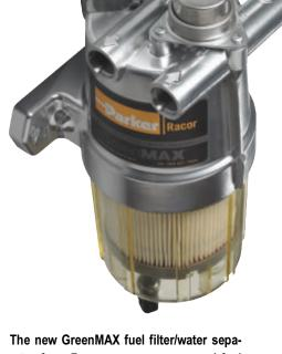
rator from Racor uses warm, unused fuel as it returns to the tank for on-demand heat transfer in cold-weather operations. This feature melts the wax and paraffin that can separate from diesel fuel at cold temperatures and can restrict fuel flow through the filters, the company said.
